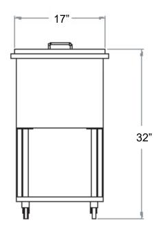
Interior Ice Basin Dimension (usable space for ice): 11"H  $\times$  14.25" D  $\times$  38" W
