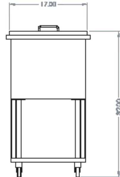
Interior Ice Basin Dimension (usable space for ice): 11"H x 14.25" D x 38" W
