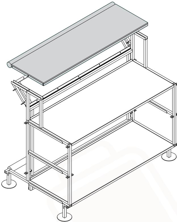
**STEP 2:** Flip and lay down counter on a flat padded surface. Counter frame facing up.
