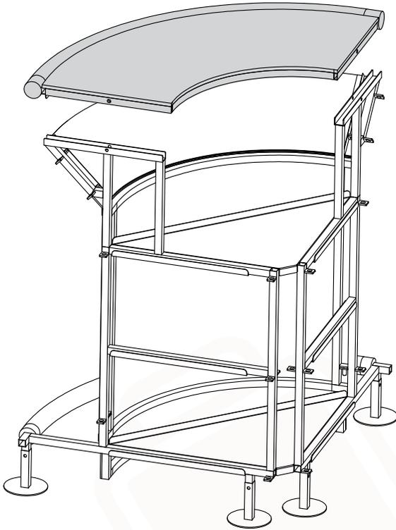
**STEP 1:** Remove lock pins and take out counter.
