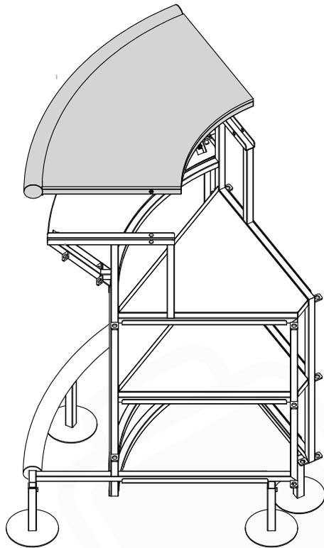
**STEP 1:** Remove lock pins and take out counter.
